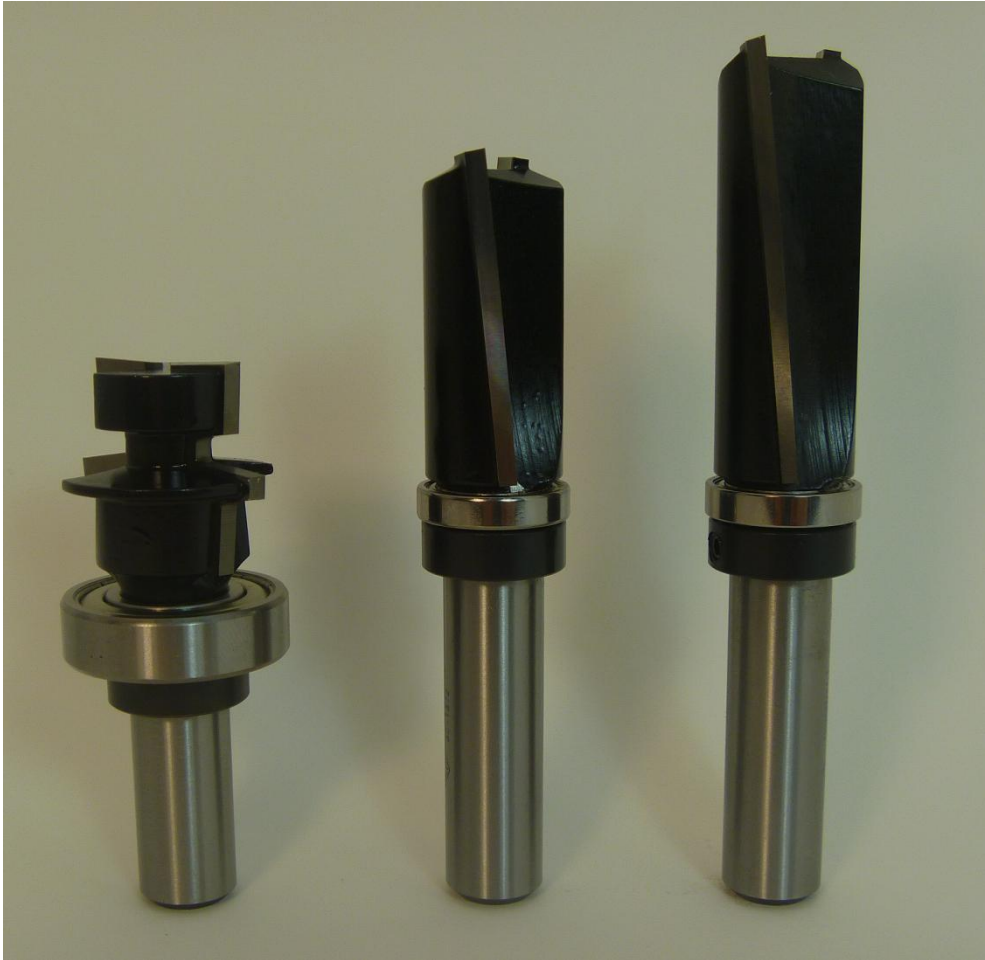
Figure 4-2. Mitre Maker cutters from left: tongue and groove , 38mm straight cutter and 50mm straight cutter
