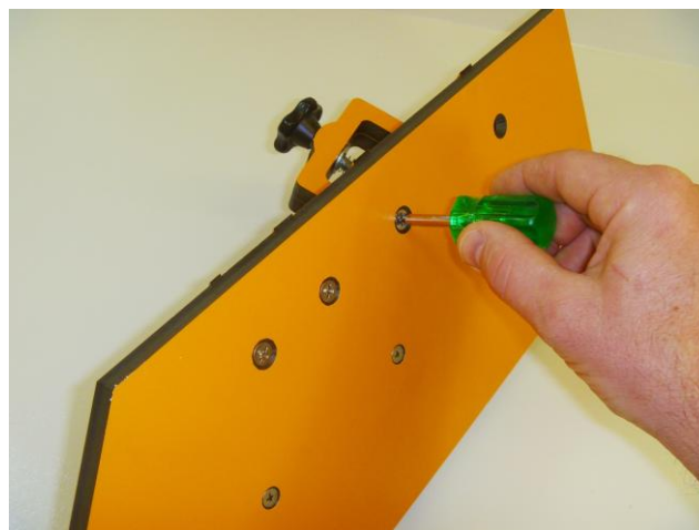
Figure 4-6. Step 4: install the fastening bolts and barrel nuts.
