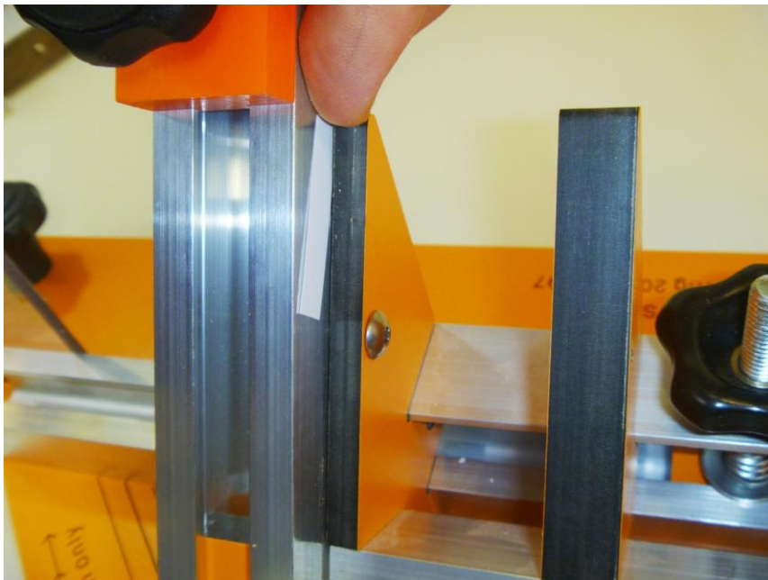
Figure 4-14. Calibration check 3: Adding a paper shim for angle adjustment
