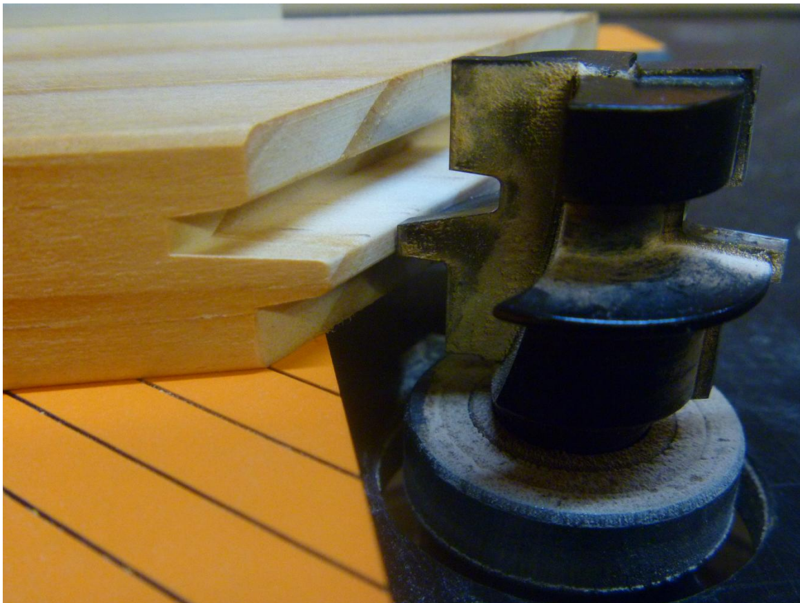
Figure 2-10. Setting the height of the tongue and groove cutter for the second half of the interlocking mitre joint
