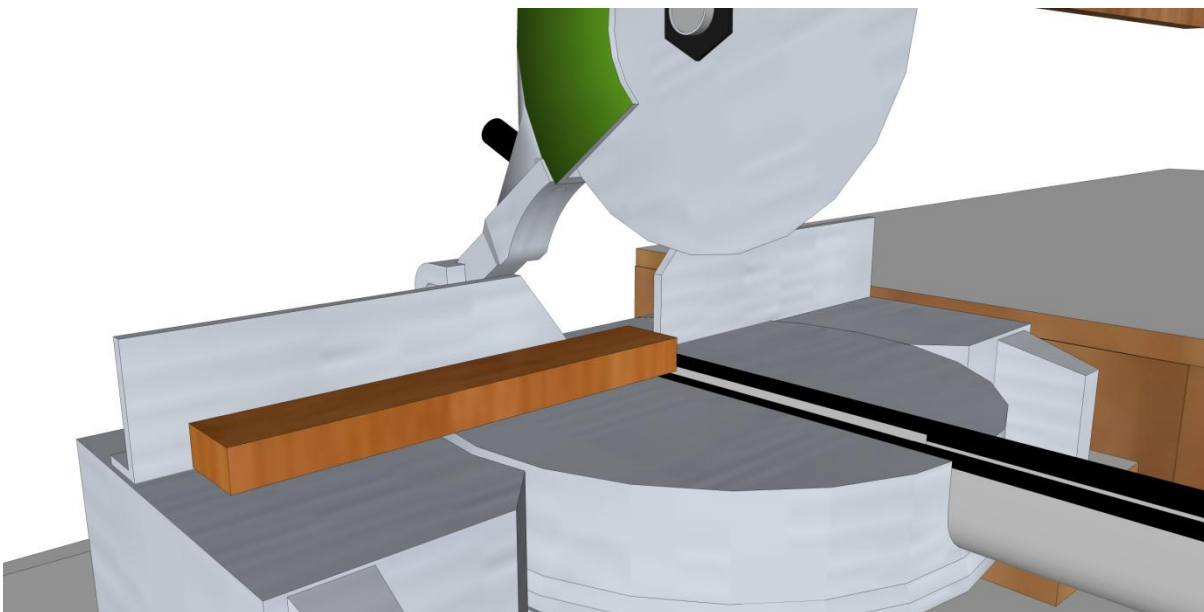
Figure 2-2. Prepare the timber: cut the timber oversize
