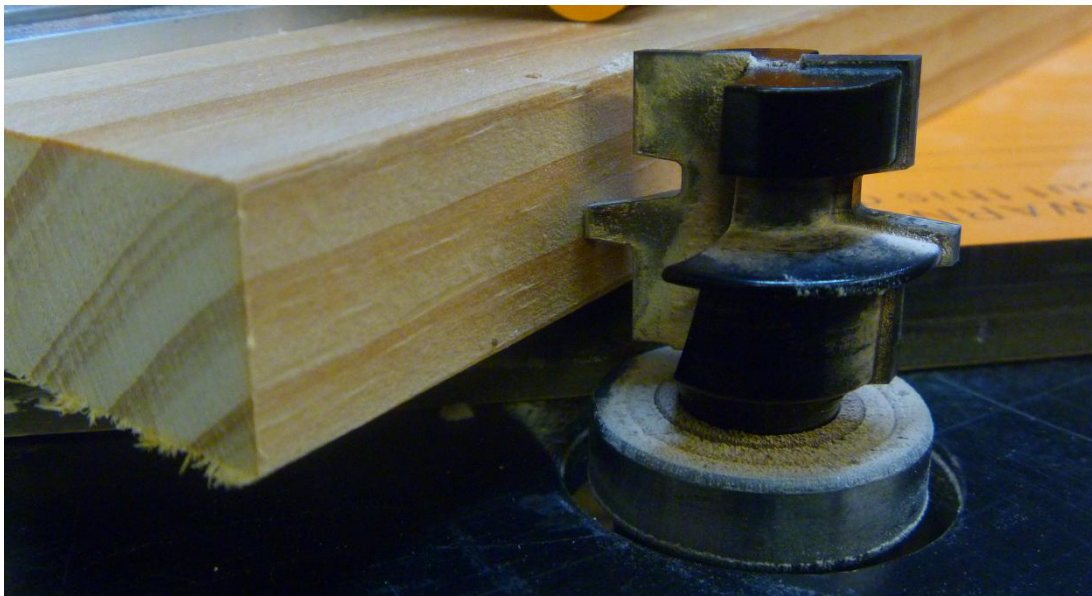
Figure 2-9. Setting the height of the tongue and groove cutter. The bearing may be partially below the table surface
