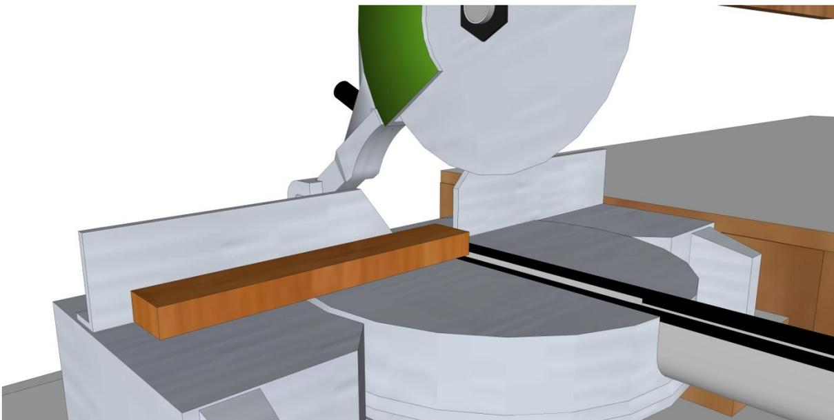
Figure 2-2. Prepare the timber: cut the timber oversize
