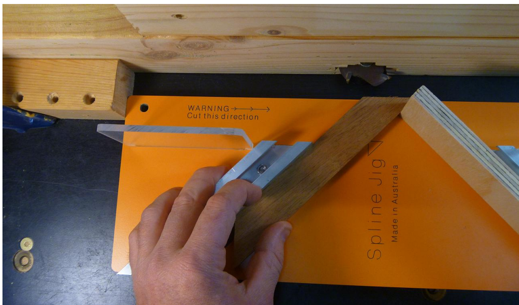
Figure 2-6. Clamp a stop block on the router table for 'hidden' spline slots
