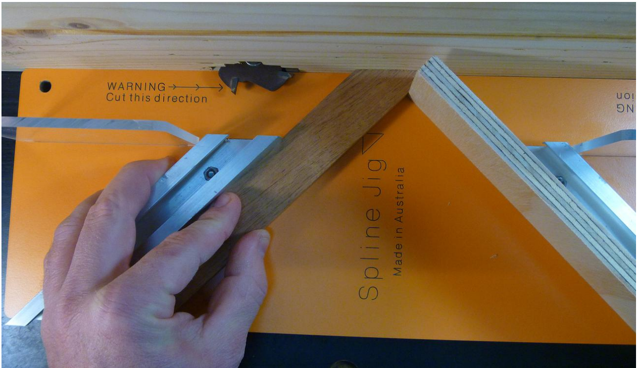
Figure 2-5. Setting up the removable fence pieces for a through spline slot in a frame corner.
