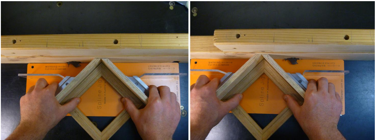
Figure 2-2. Hold the frame firmly in the jig with both hands and pass it along a fence and slot cutter so that the slot cutter moves in the direction shown the jig
