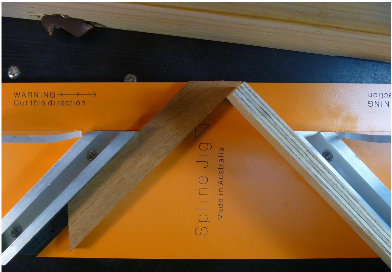
Figure 2-4. Setting up the removable fence pieces for a through spline slot in a frame corner.
