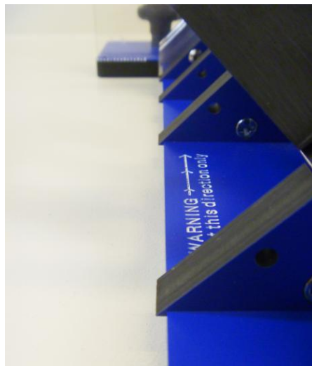
Figure 3-1. The 45 degree supports and the aluminium fence will be trimmed in the first use
